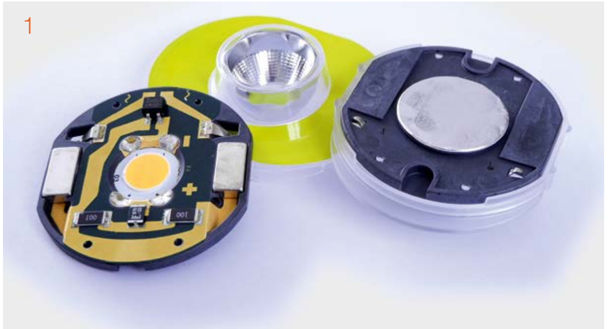
Figures 1 to 3: Examples of 3D manufactured LED modules and lamps - Clip'n Slide track system of home lights. The clips (1) – produced by means of LDS technology - simply adhere to the track via magnets (2). Placing circuit paths on any 3D metal body - the new LDS powder paint opens new opportunities in LED technology to manufacture traditional looking LED lamps (3)
