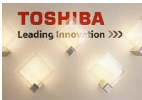
Toshiba's transparent OLED panel's unique feature is to emit light from one side only
