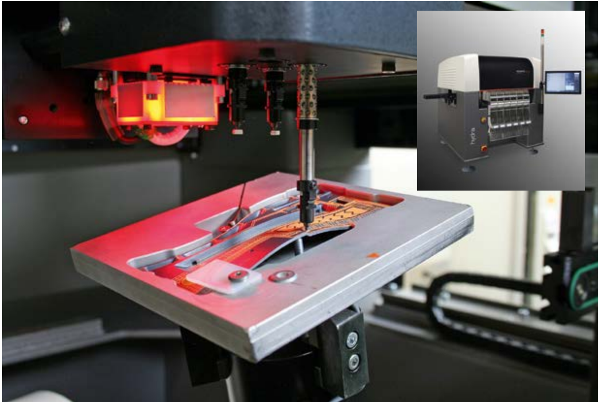
Figure 4: A view inside the assembly unit Hydra - a robot places the component in the working chamber. Inset: The assembly unit Hydra
