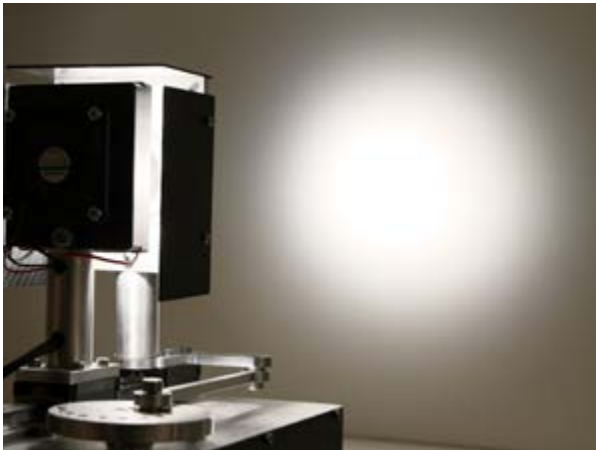
Figures 14 & 15: Zoom optics made of glass - like this one from B&M Optik - show astounding good efficiency and light distribution properties at narrow and wide angles
