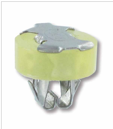
Figure 6: Consisting of a metal spring and elastic silicone, the Push-to-Fix element ensures a large area of contact between the circuit board and the luminaire housing, resulting in excellent heat dissipation
