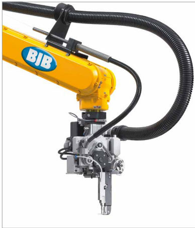
Figure 2: The wiring tool with cable feed enables precise wiring of LED luminaires even when space is extremely limited
