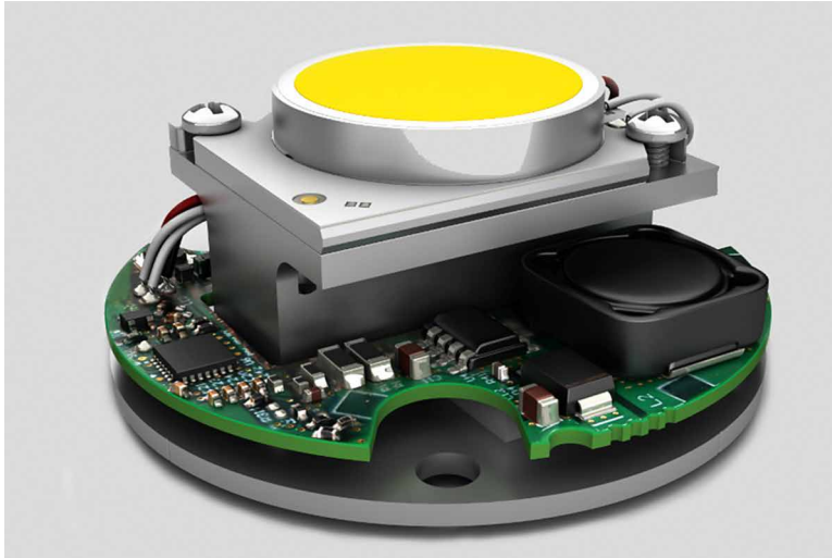
Figure 5: Experts agree that intelligent lighting modules like this Xicato XIM module that offers additional features and which can be integrated in the IoT will soon be an integral part of our technical lives
