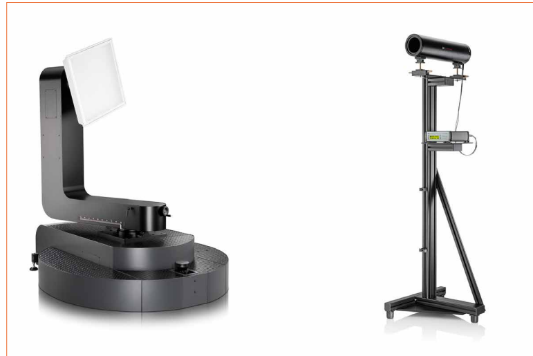
Figure 1: The goniometer in standard turning-luminaire configuration (left) and detector with stray light tube on stand (right)
