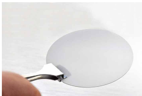
According to research results, using semi-polar GaN has the ability to reduce droop in blue LEDs
