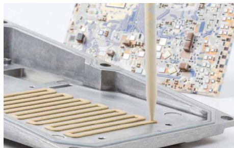
The heat-conducting SEMICOSIL® 961 TC silicone filler from Wacker is applied directly to the heat sink. Once the electrical circuit is pressed on, the gap filler cures to form a soft, cushioning silicone layer that optimally transfers heat to the heat sink
