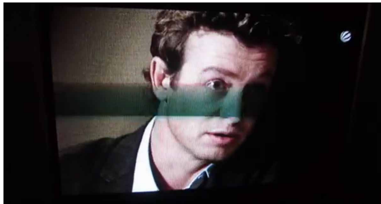
Figure 3: Photos from CRT TV monitors show the 25/50 Hz flicker as banding. An effect that appears very similar when taking pictures or videos using flickering LED lamps
