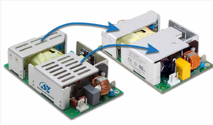
Figure I: Use solid heat-sinks to add more contact area with cold plate
