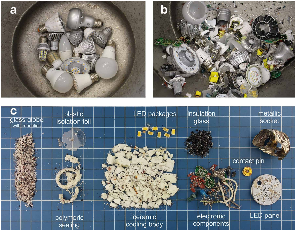
Figures 7a-c: (a) Mix of waste LED lamps prior to EHF. (b) Component and material mix obtained after EHF of the waste lamps shown in a. Here, a very coarse fragmentation was aimed at (c) Fractions obtained after EHF of one single retrofit lamp and subsequent manual sorting
