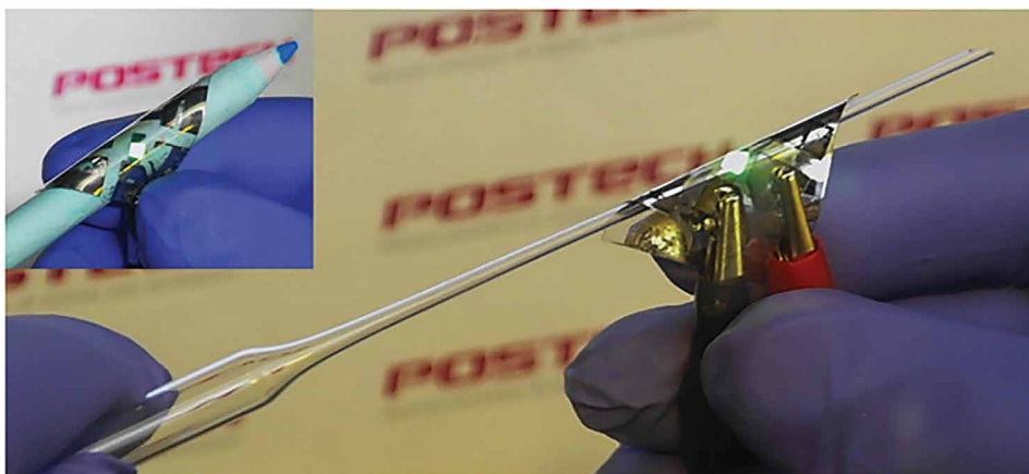
OLEDs with a graphene anode wrapped on cylinders with different curvatures
