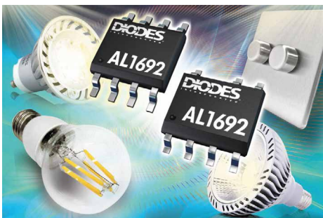
Diodes AL1692 controller-only version is offered in an SO-8 package while the MOSFET options are supplied in an SO-7 package
