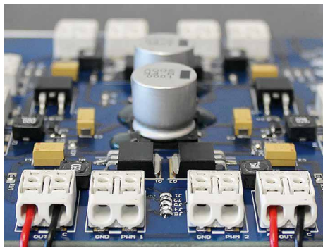
Electro Terminal has developed the Microcon SMD Power connector to provide direct mains voltage supply to electronic PCBs within a lighting system
