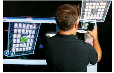
Augmented reality is used to simplify the provisioning process and ease control of lighting devices
