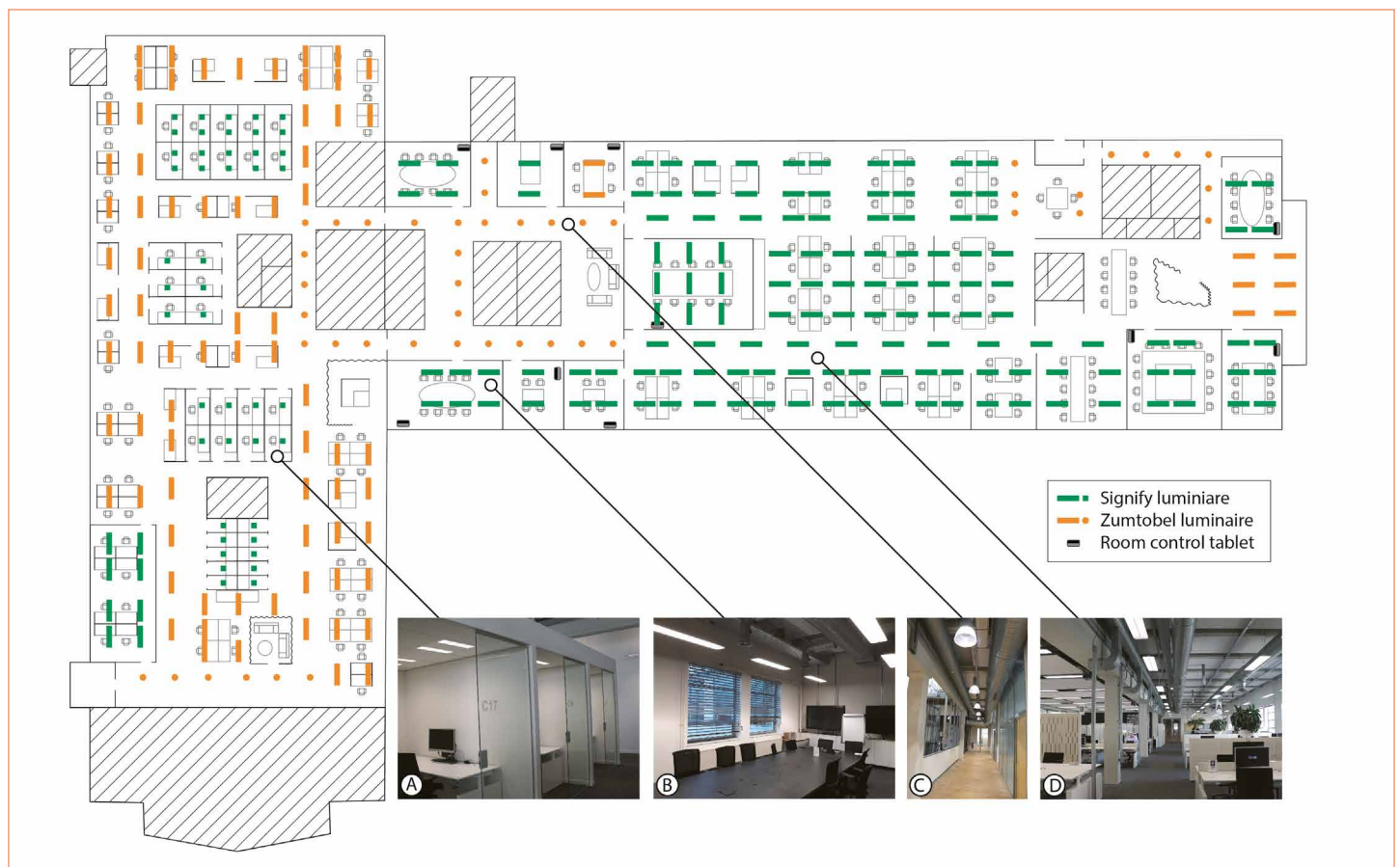
Figure 1: Floorplan of the office and photos of the different workplaces: (A) individual office; (B) meeting room; (C) corridor; (D) open office
