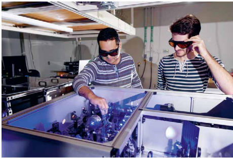
Carlos Silva (l.) in his lab with graduate research assistant Félix Thouin examining a setup to process laser light in the visible range for the testing of quantum properties in a halide organic-inorganic perovskite (Credits: Georgia Tech / Rob Felt)
