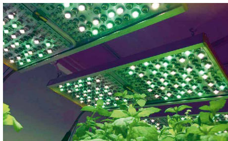
Use of Phytogy RL allows the researchers to evaluate the most varied light recipes, without having to change luminaires between individual tests (Picture credits: Osram)
