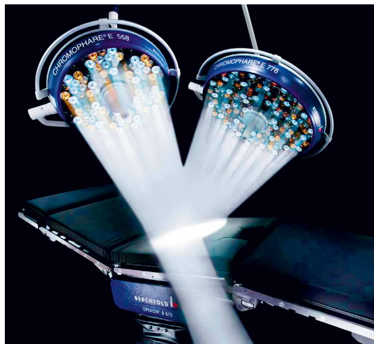
Figure 2: Stryker Berchtold Chromophare E558/E778 Surgical Light. The SLS combines separate optical modules based on high-performance LEDs and a two-stage optical system and a central reflector. Color mixture is realized by superposing the light cones on the surgical field with adjustable CCT between 3,600-5,000 K [4]
