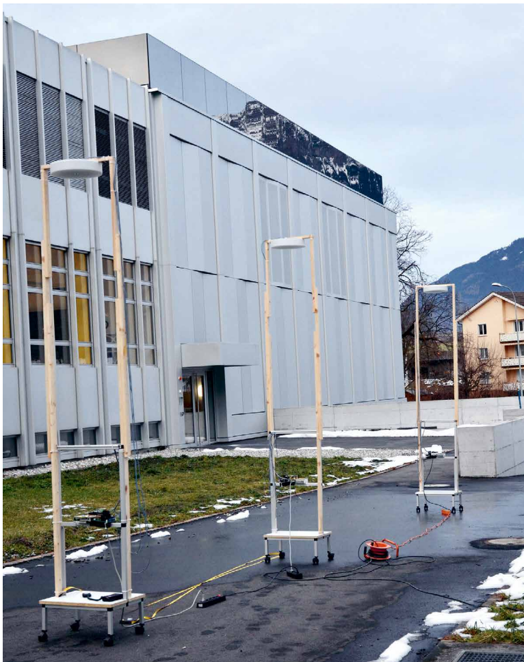
Figure 9: Example of outdoor test of the luminaires
