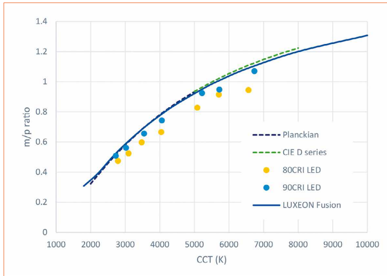
Figure 7: Melanopic to photopic ratio (tracing the blackbody locus) as a function of CCT. The new technology closely reproduces the melanopic content of daylight (CIE D series) at cool-white color temperatures while enabling lower melanopic content at warm-white color temperatures
