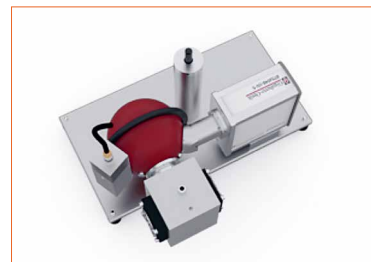
Figure 5: Example measurement system for permanent fluorescence-free measurements
