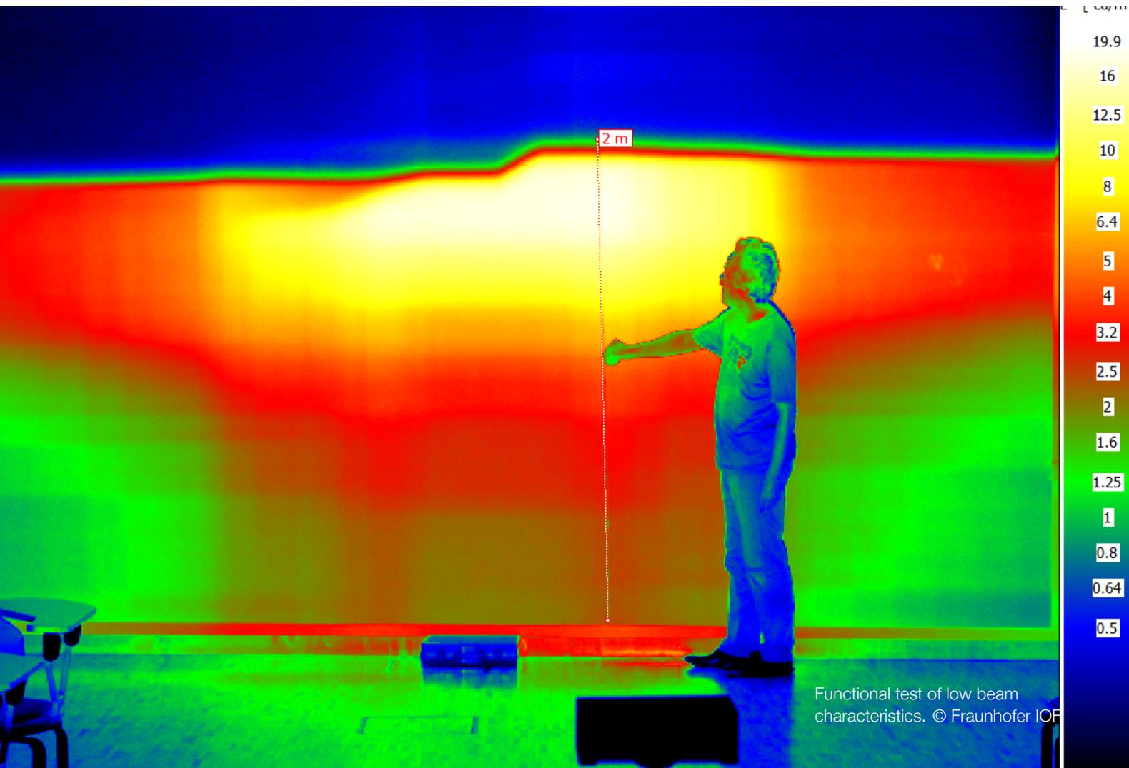
Functional test of low beam characteristics. © Fraunhofer IOF
