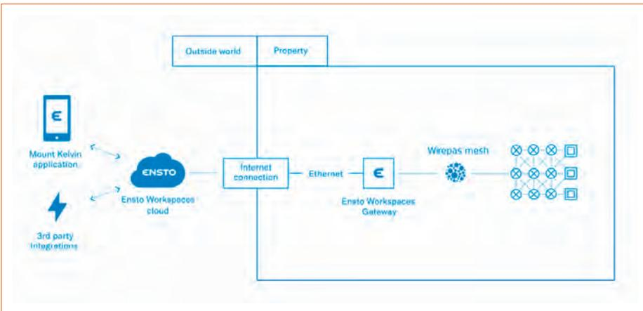
Figure 2: Example of options to connecting to the mesh network solution
