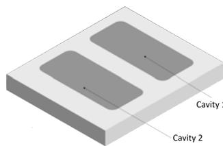
Figure 6: A tunable LED concept in one package with two separated cavities, one for cool white and one for warm white
