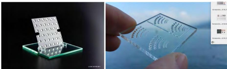
Figure 7: Digital fabrication of micro-lenses (courtesy of LUXIMPRINT)
