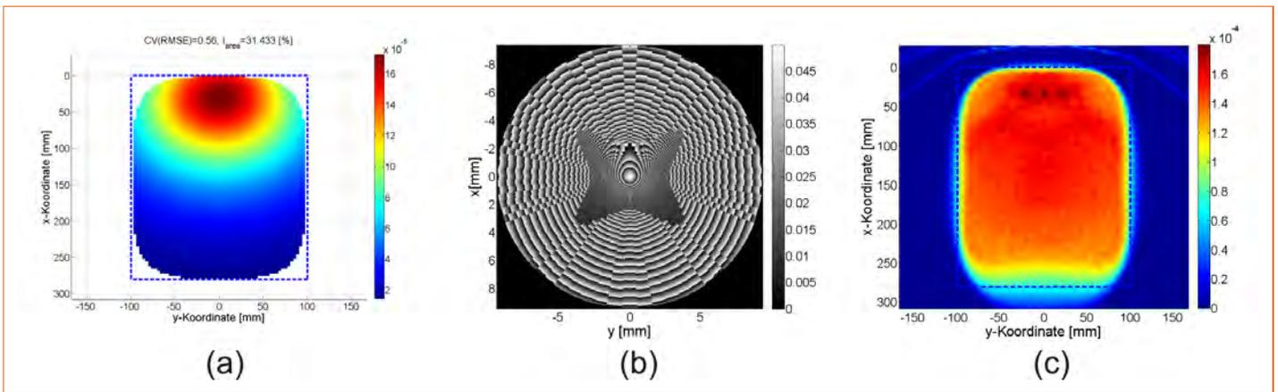
Figure 2: a) Simulated irradiance distribution within the oval shaped target area without FF-MOE. b) Calculated structure of the FF-MOE with a maximal height of 50 $\mu$ m. c) Simulated irradiance distribution within the oval shaped target area with FF-MOE
