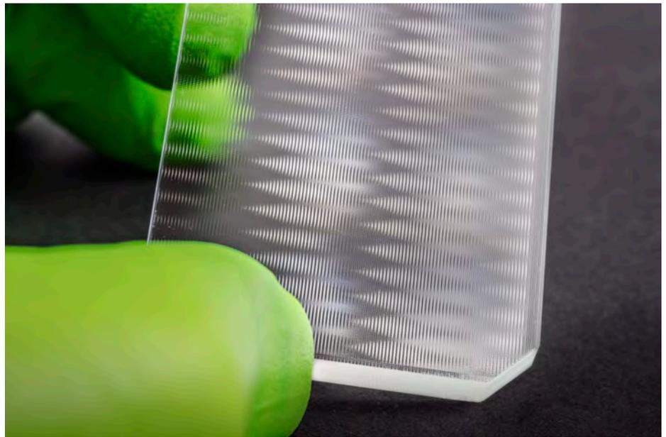
Figure 1: Replicated high-beam micro-optics (iFEC structure). © Fraunhofer IOF
