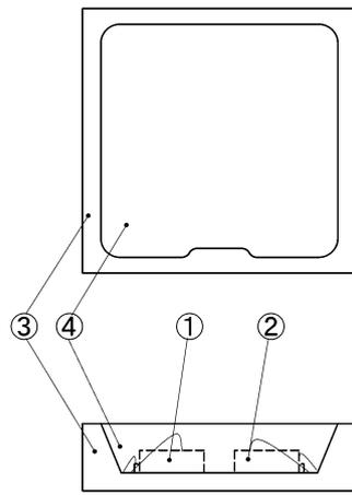
Figure 5: Internal structure of the 2-in-1 package
