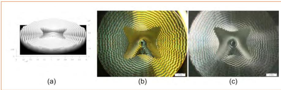
Figure 3: a) 3D Model of the calculated FF-MOE. b) Light optical microscope images of the master structures of the calculated FF-MOE, manufactured using the MALA-System. c) Light optical microscope images of imprinted FF-MOE structures on a PMMA substrate
