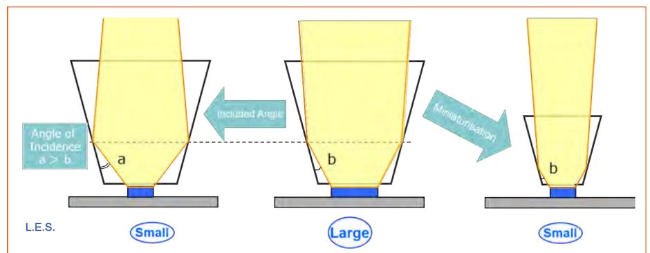
Figure 7: An example of how a spot design can be improved, or optimised for size.
