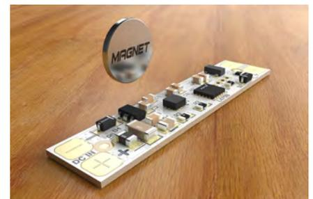
Cezos' new magnet switch, L475T, with its ultra-low-power high-performance three-axis magnetic sensor offers many useful features for its applications like inside cabinet LED lighting
