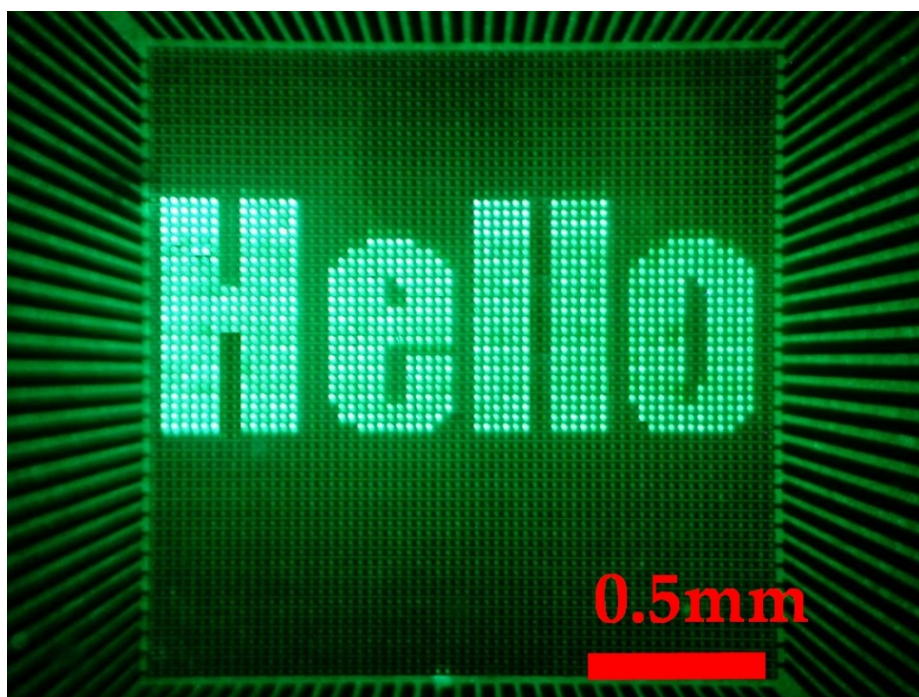
Figure 4: Plan view optical micrograph image of a green-emitting 128x128 matrix-addressable micro-LED array.
