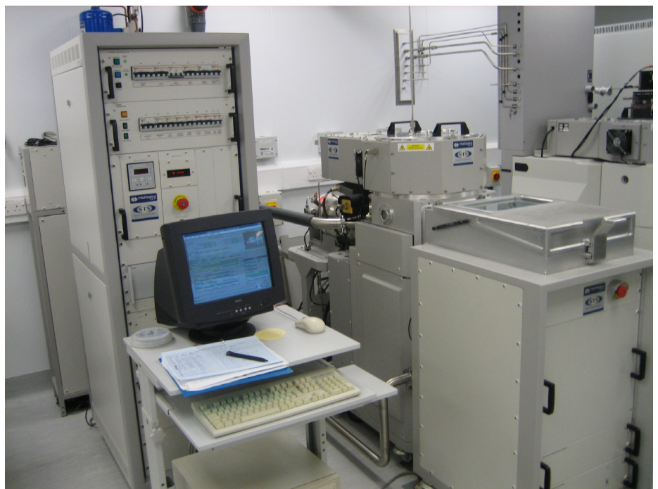
Figure 9: Part of the Institute of Photonics cleanroom showing ICP dry etching tools essential for micro-LED research.
