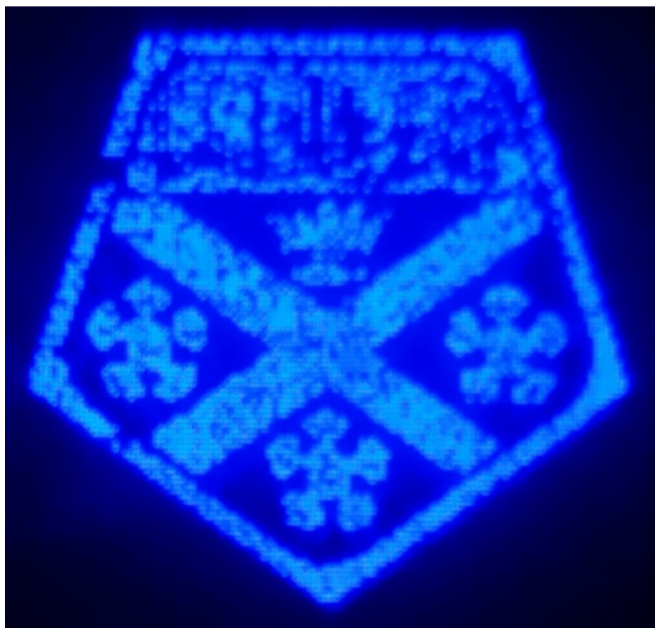
Figure 5: Plan view optical micrograph image of a blue-emitting 128x128 active-matrix micro-LED display, showing the University of Strathclyde crest. This chip is capable of up to 1 Million frames per second update rates.
