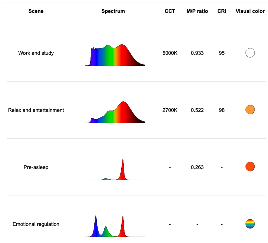
Figure 3: Spectrial recipes for the different lighting scenes based on Yuji LED components.
