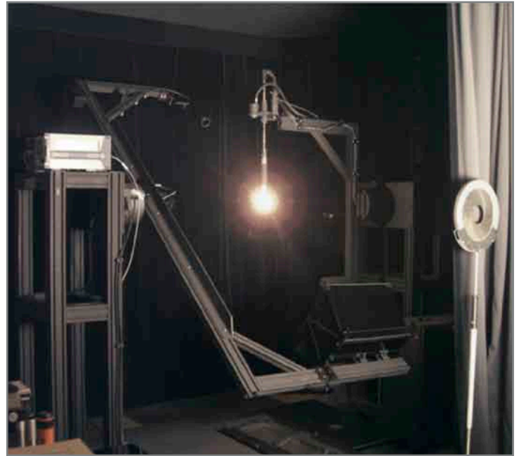
Figure 5: NIST gonio-spectroradiometer for the total spectral radiant flux scale realization
