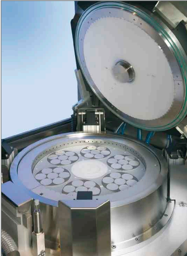
Figure 2: Planetary Reactor® AIX 2800G4 HT in 42x2" configuration for blue, green or white LEDs
