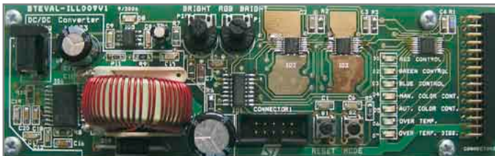
Figure 3: Demonstrator board STEVAL-ILL009V1
