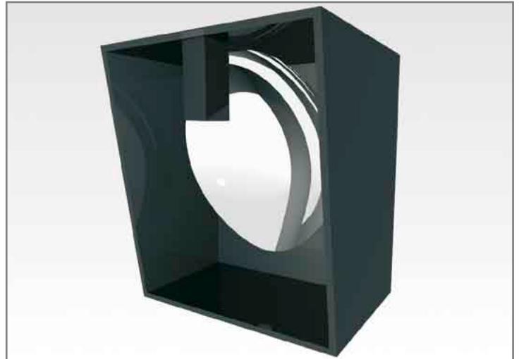
Figure 6: Luminaire with 3D tailored free-form mirror. The LED with mixing optics is integrated in the little vertical bar. The free form mirror is tailored to yield uniform illumination across an area of 2 m by 1 m
