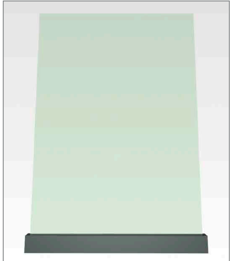
Figure 3: Light guide of 30cm x 20cm in minimalistic design. It is illuminated from the lower side by RGB LEDs
