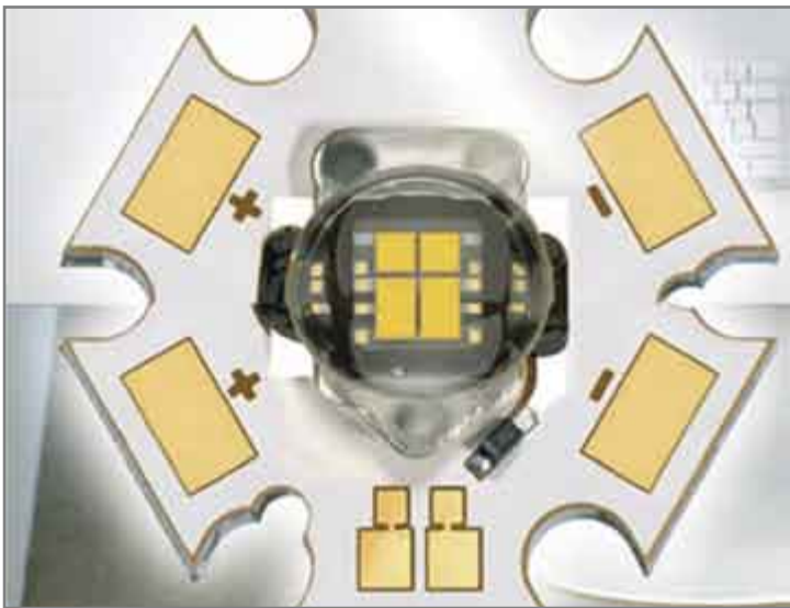
Figure 1: Example of a series string of LEDs in one package (OSRAM Ostar).
