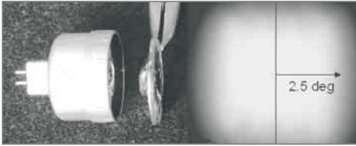
Figure 7: Left: Photo of a "Chip LED bulb replacement"2. An identical RXI as mounted in the housing is held in front of the full assembly. Right: Radiation pattern of the RXI with a green Luxeon LED. The vertical bars visible in the pattern are caused by the contacts of the LED chip.
