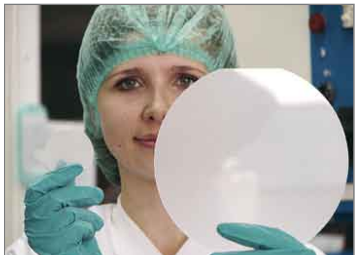
The 8" sapphire wafer has 16 times the face of a standard 2" wafer.
