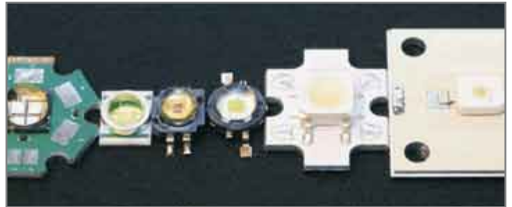
Figure 2: LEDs as light sources vary much from each other. The same optics cannot be used for several LEDs without jeopardizing the performance.
