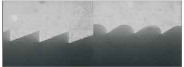
Figure 23: Side by side comparison of fidelity when molding microprism facets with: Left: compression molding and Right: injection molding.
