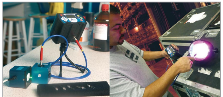
Figure 6: Portable spectrometer measuring single LEDs(left) that will be used for entertainment light fixtures as the one shown at a concert hall on the right photograph
