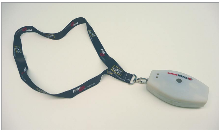
Figure 7: Handheld spectrophotometer with the latest advances in wireless communications and compatibility with other common handheld devices such as the iPhone
