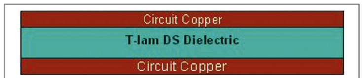
Figure 3: T-lam DS Substrate Illustration.
