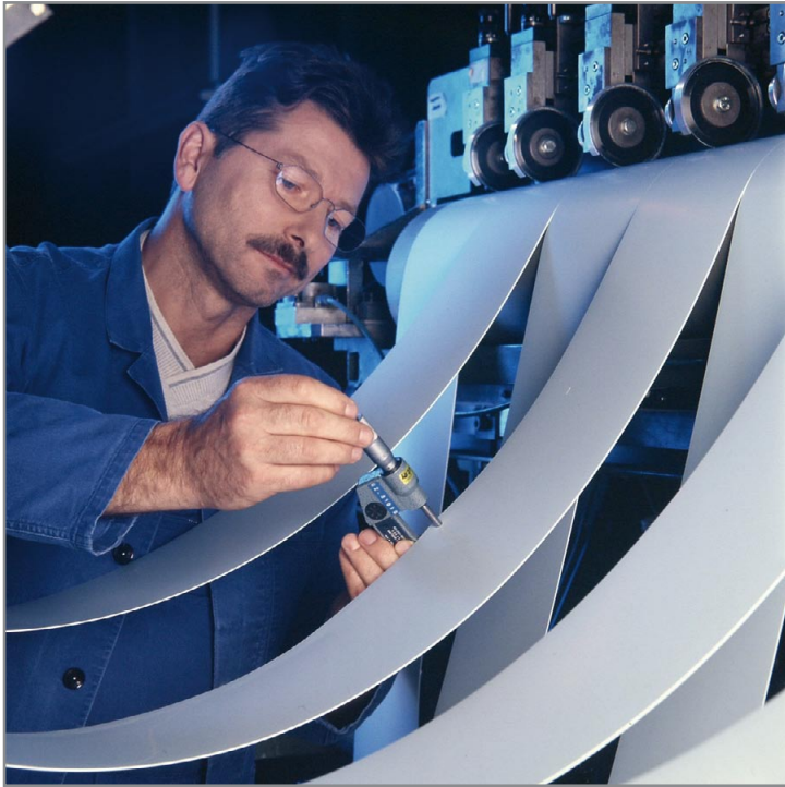
Figure 6: Film casting lends itself to the manufacture of thin ceramic disks. The surfaces are remarkably smooth, with thicknesses ranging from 0.1 to 1.5 mm. Further processing is done by punching and laser treatment.
