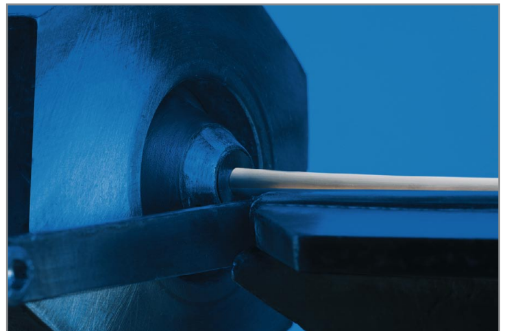
Figure 9: Extrusion is an economically viable process for mass production of rotationally symmetrical components such as rods and pipes. Lengths from 3mm up to 400mm are possible. The diameters for rods range from 0.5mm to 20mm, and in pipes diameters up to 40mm can be produced.
