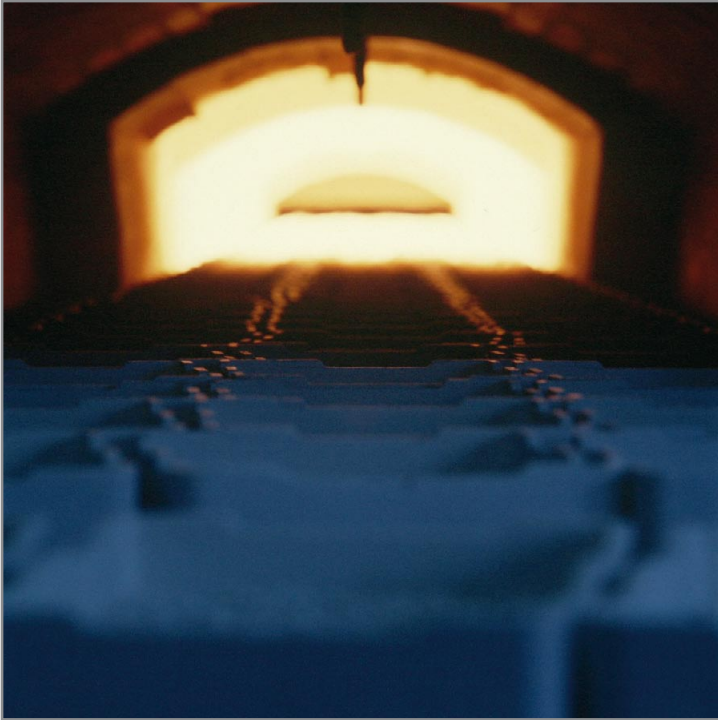
Figure 10: Sintering is a process where the formed parts undergo a heat treatment below the melting temperature.
