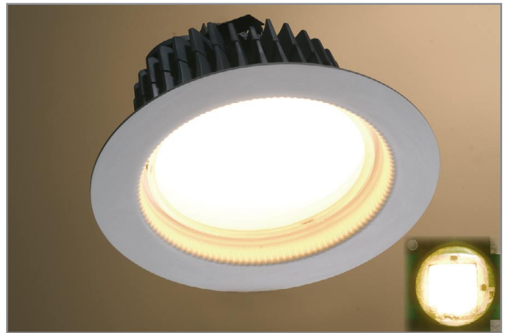
The high-efficiency LR6 prototype features TrueWhite™ technology, resulting in a 92 color rendering index and a 3500K color temperature by using the latest Cree LEDs, the XLamp® XP-G.
