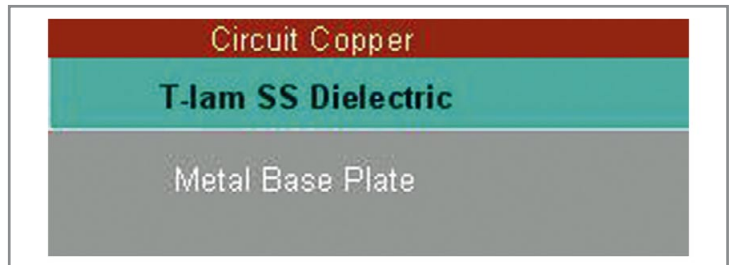
Figure 2: T-lam SS Construction.
