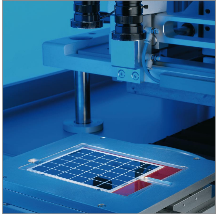
Figure 11: In a final step before the final inspection metallization pads and electrical circuit tracks are applied.
