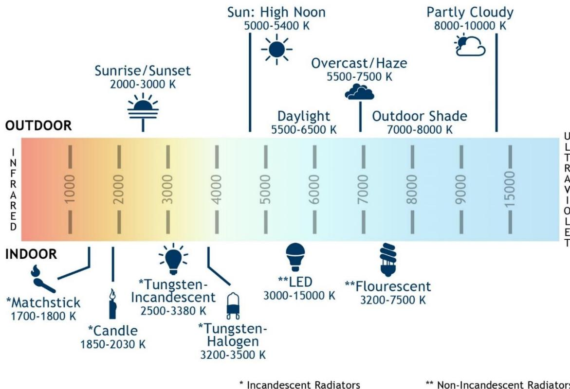
**Figure 7** – Comparing the CCT of various light sources, including sunlight at different times of day and weather conditions, and indoor artificial light sources. Sunlight above the atmosphere is approx. 5900 K. As the Sun crosses the sky, it may appear red, orange, yellow, or white, depending on its position. The changing color of the Sun throughout the day is mainly the result of light scattering by atmospheric gas molecules.
