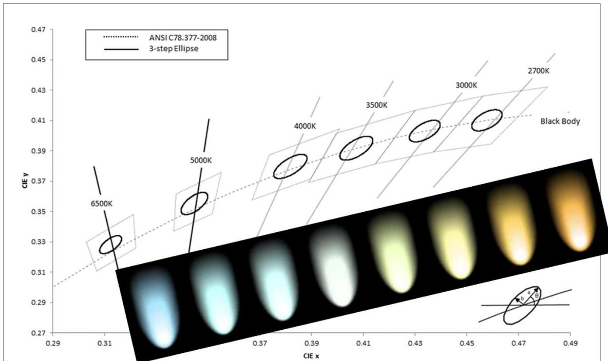
**Figure 12** – Illustration of how light at different CCT levels appears to the human eye - “cool” blue at 6500 K, and “warm” yellow-orange as light moves into the 3000 K range and below.<sup>†</sup> Shown correlated with CIE coordinates.
