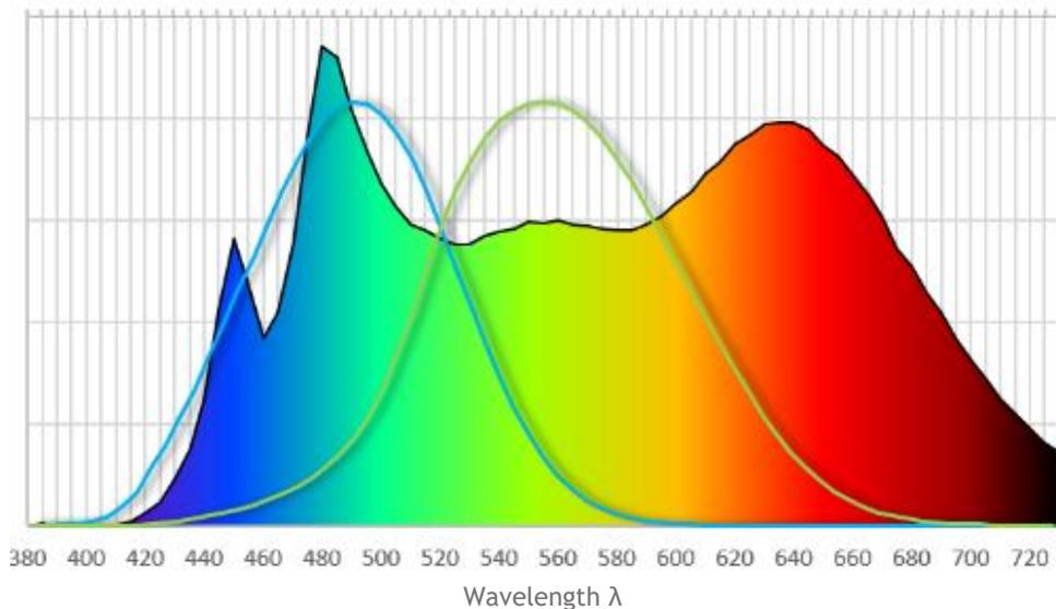
**Figure 14** – The SPD of a 4000 K Salud LED, shown with circadian (blue) and visual (green) response curves. Salud LEDs provide sufficient red light for accurate skin-tone rendering and fill the cyan gap for enhanced melanopic spectral content.
