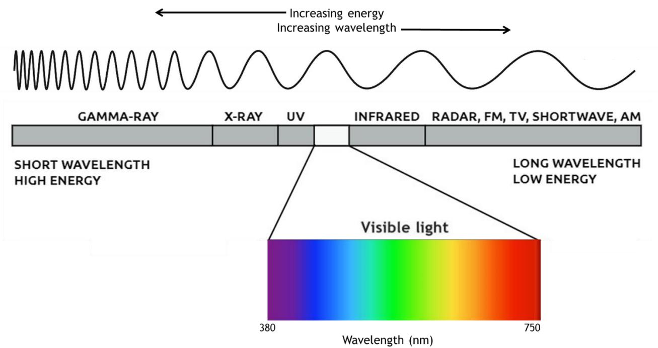
**Figure 4** – The spectrum of electromagnetic radiation, including invisible wavelengths such as X-rays and radio waves, plotted in order of increasing wavelength (in meters). The bottom bar is an expanded view of the visible light spectrum, the narrow range of electromagnetic radiation that the human eye can perceive, from roughly 380 nanometers (nm) to 750 nm.
