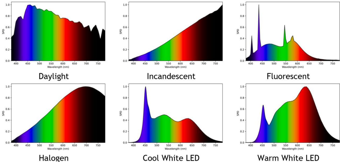
**Figure 8** – A comparison of SPDs for different white light sources demonstrates that daylight (represented here by the SPD of typical winter morning light in the Northern Hemisphere, upper left) offers the broadest spectrum. Red wavelengths dominate incandescent bulbs, for example. You can design LEDs to offer a wide range of different white color temperatures. (Image Credit: Admesy)
