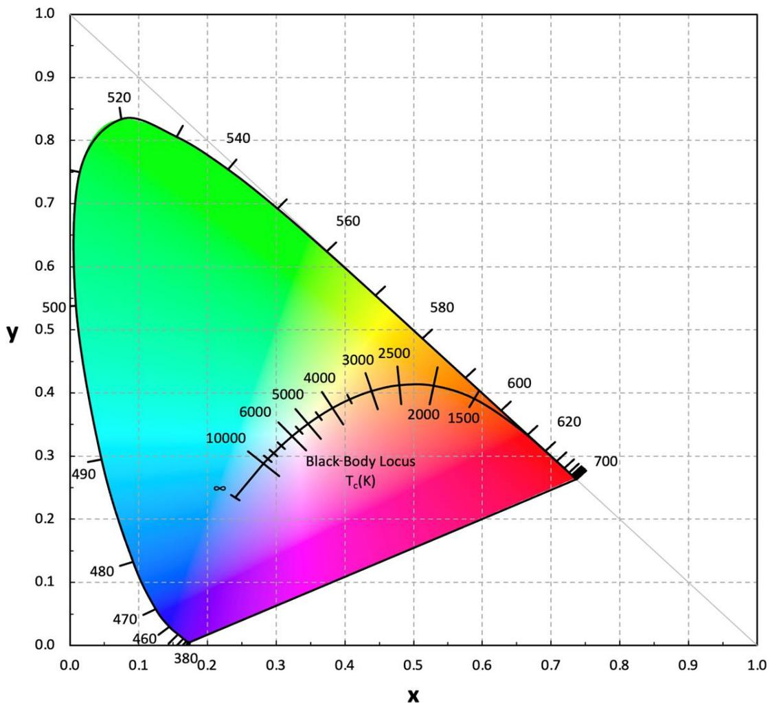
**Figure 6** – A graphical representation of the CIE 1931 color space, charting all colors visible to the human eye. Numbers around the edge of the “horseshoe” are wavelengths of monochromatic light defining the boundaries of the color space. Inside the horseshoe, each perceptible color has a coordinate called CIE<sub>x</sub>, CIE<sub>y</sub>. The black body (Planckian) locus coordinates are shown, T<sub>c</sub>(K); the black-body temperature, is commonly called CCT.
