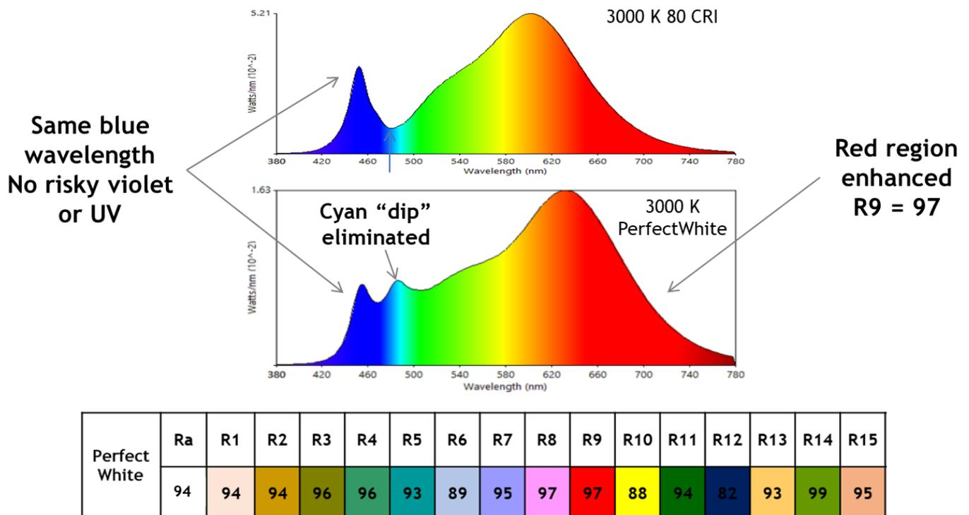
**Figure 9** – The two graphs show that Luminus PerfectWhite LEDs correct the cyan gap (compared to a typical 3000 K LED with CRI of 80), providing more balanced, full-spectrum light. The values in the table show the excellent CRI performance of PerfectWhite with an average value (Ra) of 94.3 (out of 100) on the 15 color samples (R1-R15).
