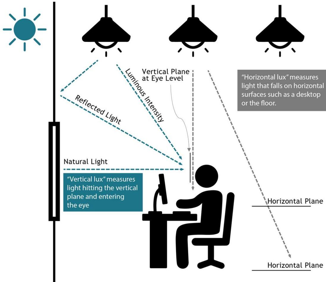
**Figure 13** – Traditional lux is horizontal: measuring light falling on a flat surface. HCL considers both horizontal and vertical lux, which is light measured on the vertical plane in front of the human occupant and at their eye level. The WELL Building Standard guidelines on circadian lighting [4] assume eye level is 1.2 m or 4 ft above the finished floor level.
