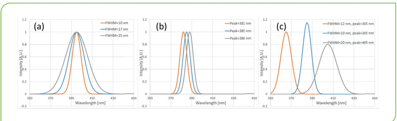
Figure 4. Different LED spectra to be measured with irradiance sensor
