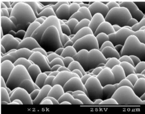
SEM view of a Light shaping Diffuser surface microstructure.
