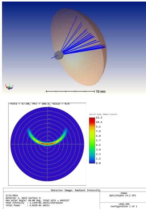
**A basic example using Luminance LSD scatter function in OpticStudio. Notice that the input ray angle is highly oblique from the surface normal.**
