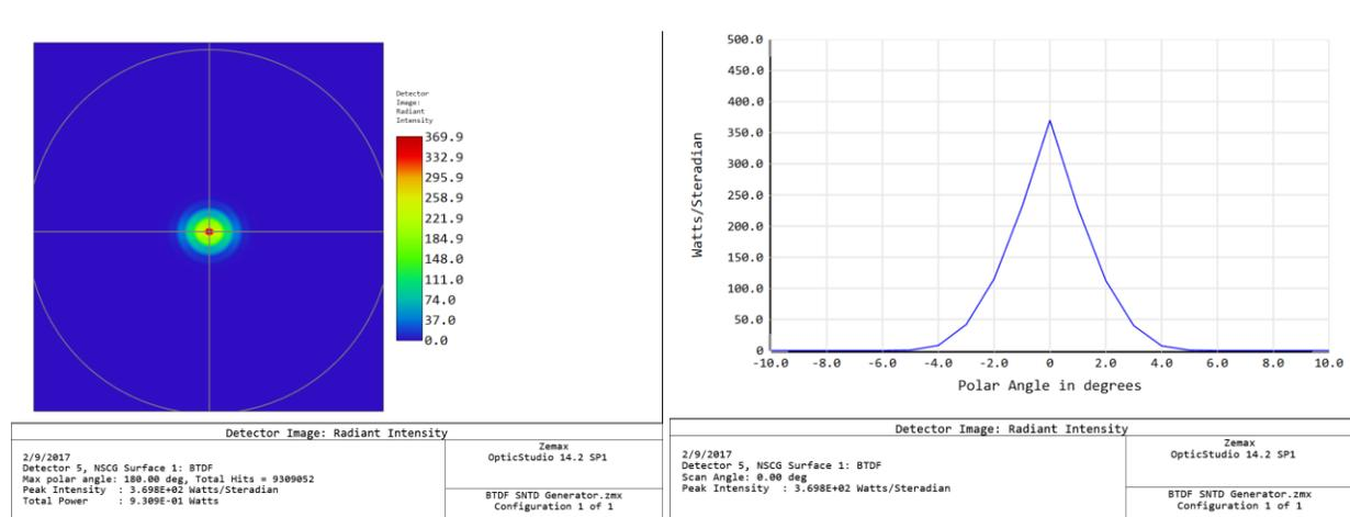
**$1^\circ$  Diffuser profile with 1 degree resolution**
